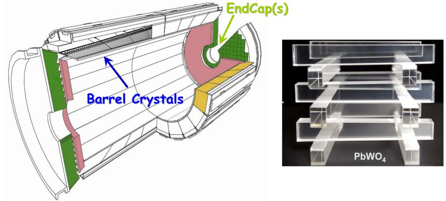
Barrel: 61,200 crystals in 170  $\varphi$ -rings of 360 ( $|\eta| < 1.48$ ) Two Endcaps: 7,324 crystals each (1.48< $|\eta| < 3$ ) Test beams: energy resolution of <0.5% (~100 GeV e<sup>-</sup>) Goal: achieve and maintain it in situ at the LHC !
